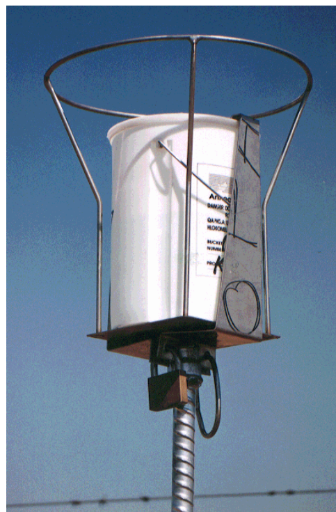
Figure 2 Single bucket monitoring unit, showing sampling bucket with bird ring and security clamp.
